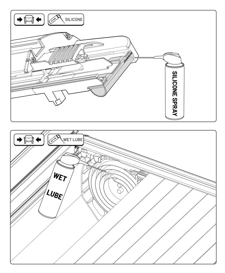
• Regularly, and following cleaning, spray the inside of the canister ends with a PTFE free all-conditions wet lube product.
