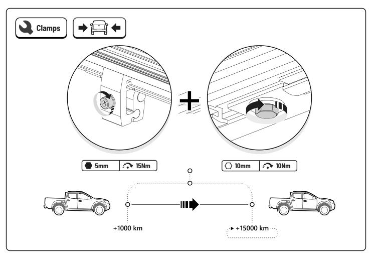
• Re-tighten the clamps to 15 Nm 1000 km after first use. And then every 15.000 km
