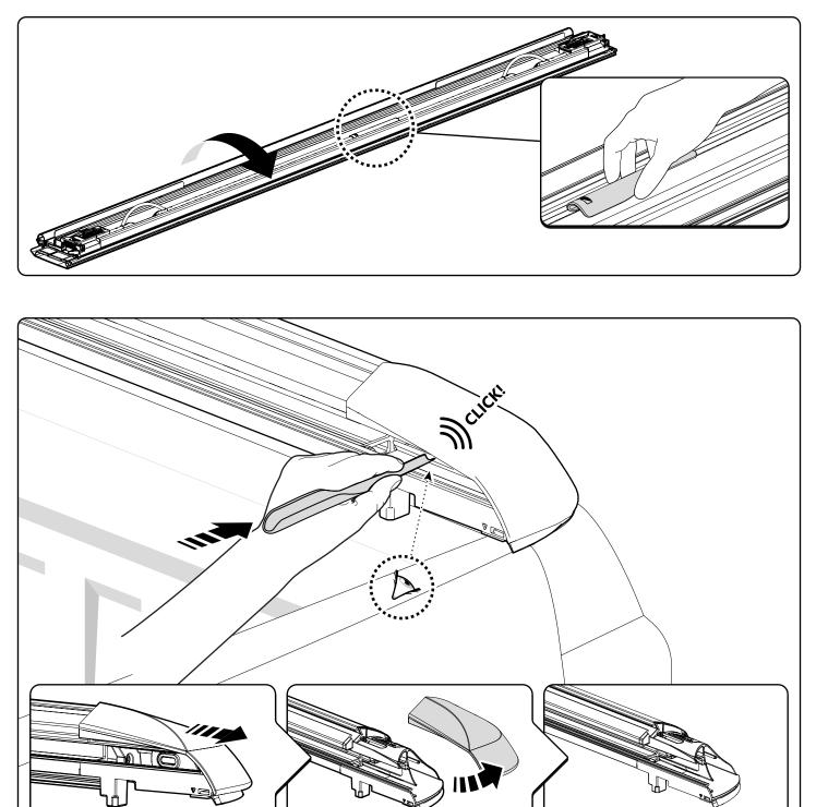
• Use the multi tool to remove the plastic covers on the side profiles.
