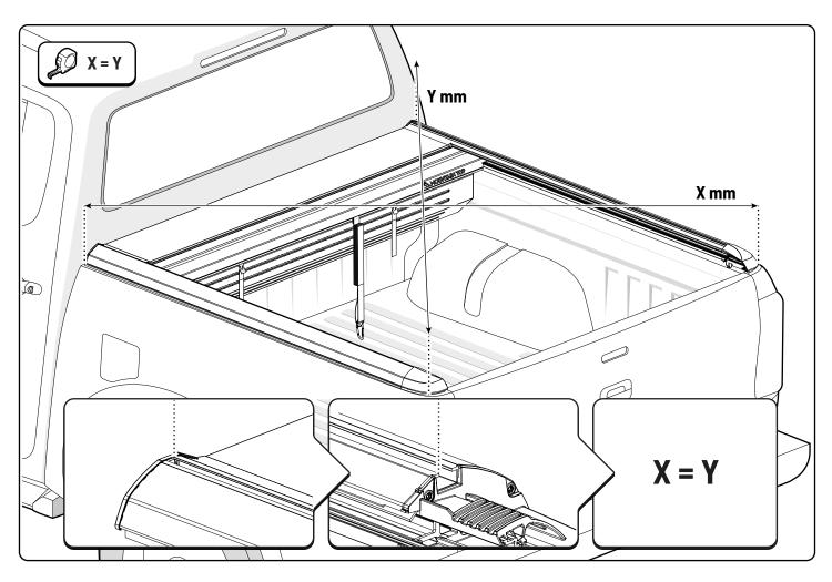
• Ensure the cross measurements are identical.
